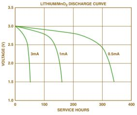
Figure 1. Typical discharge curves.
