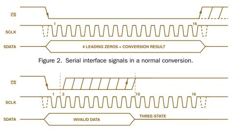
Figure 3. Using the serial interface signals to enter power-down mode.
