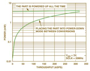
Figure 5. AD7476A power consumption comparison.
