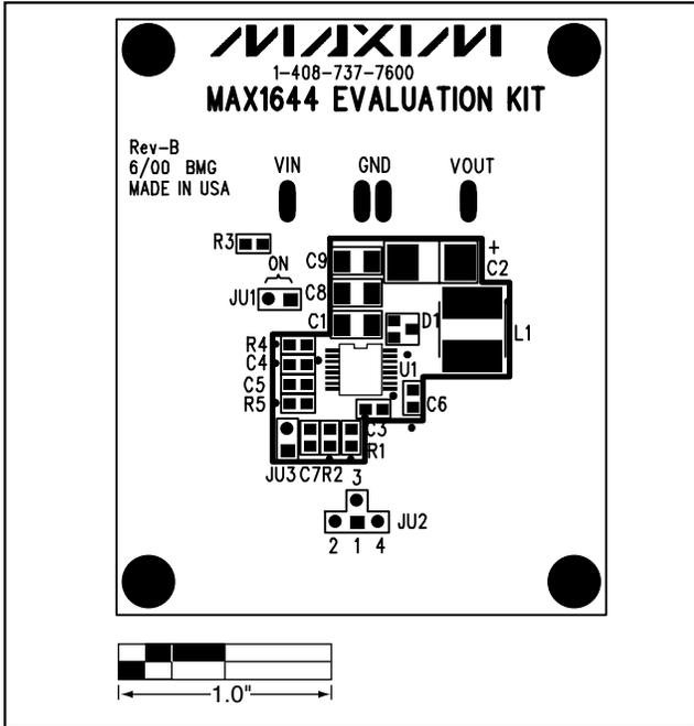
Figure 2. MAX1644 EV Kit Component Placement Guide—Component Side
