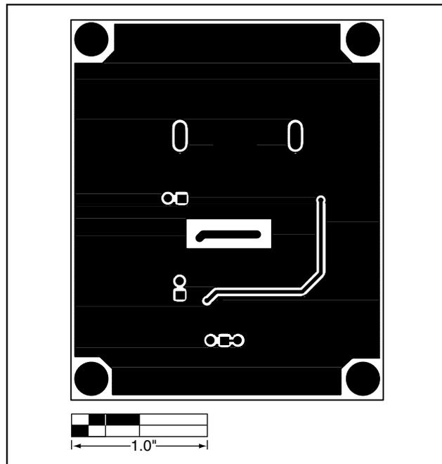
Figure 4. MAX1644 EV Kit PC Board Layout—Solder Side
