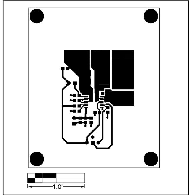
Figure 3. MAX1644 EV Kit PC Board Layout—Component Side
