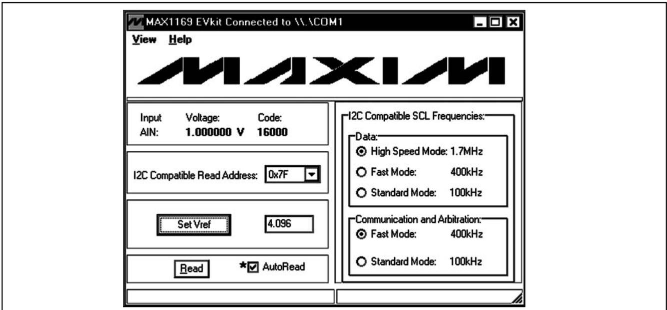
Figure 1. Main Window of the MAX1169 Evaluation Software
