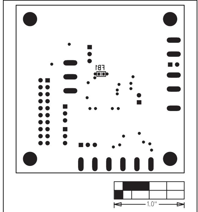
Figure 8. MAX1169 EV Kit Component Placement Guide—Solder Side
