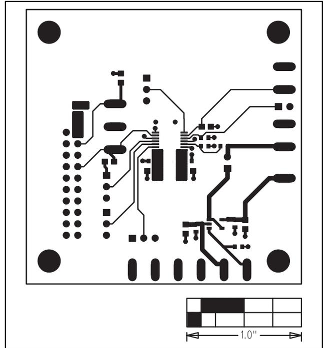
Figure 4. MAX1169 EV Kit PCB Layout—Component Side
