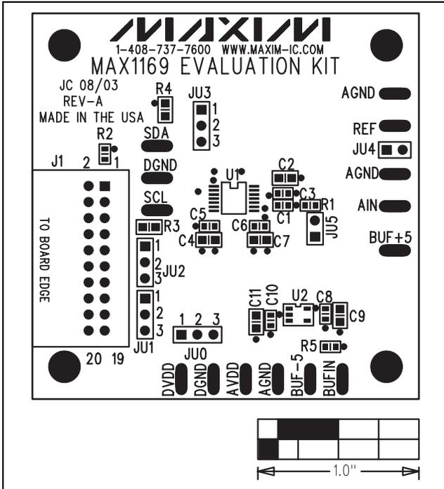
Figure 3. MAX1169 EV Kit Component Placement Guide—Component Side
