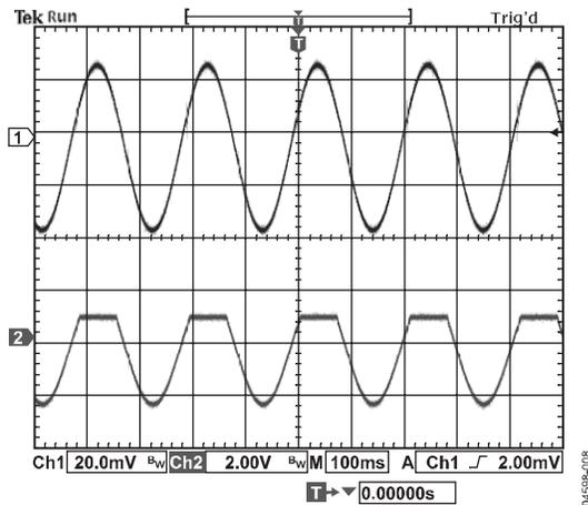
Figure 12. Response with  $V_{CLAMP}$  Set
