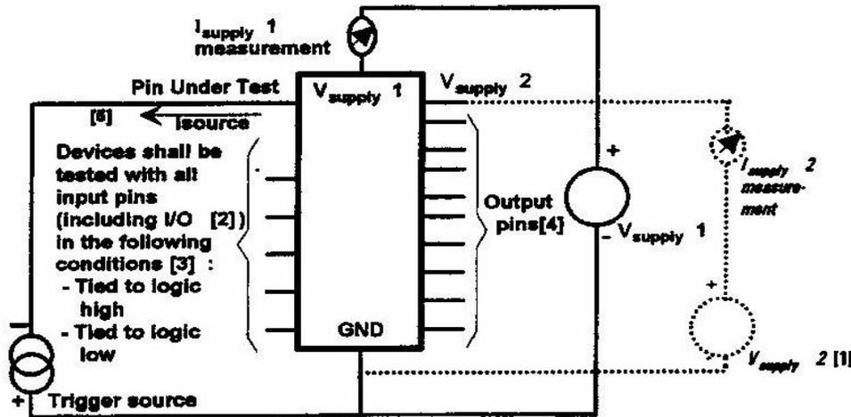
1. DUT biasing shall include additional  $V_{supplies}$  as required.
