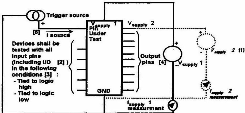
1. DUT biasing shall include additional  $V_{supply}$ s as required.
