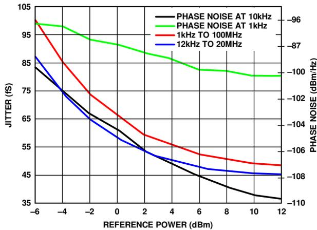
Figure 34. Jitter and Phase Noise,  $f_{\text{PFD}} = 100 \text{ MHz}$
