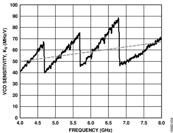
Figure 40. VCO Sensitivity,  $K_V$  vs. Frequency  $VCC\_VCO = 3.3 V$
