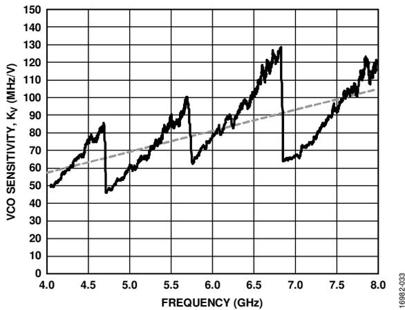
Figure 39. VCO Sensitivity,  $K_V$  vs. Frequency  $VCC\_VCO = 5 V$
