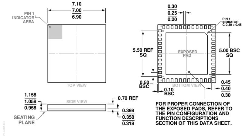
Figure 45. 48-Terminal Land Grid Array Package (LGA)
