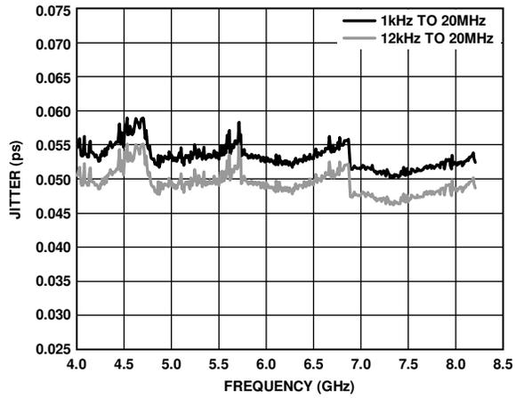
Figure 27. RMS Jitter, Fractional-N,  $f_{PFD} = 153.6$  MHz,  $VCC\_VCO = 5$  V
