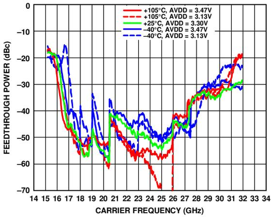
Figure 25. RF32P and RF32N VCO  $\times$  5 Feedthrough, De-Embedded Board and Cable Measurement, Combined Using Balun
