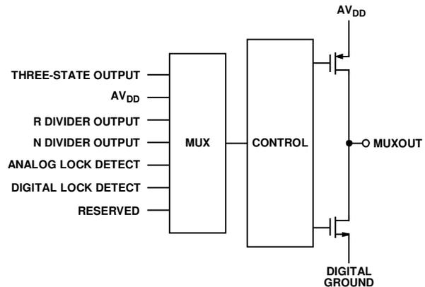
Figure 38. MUXOUT Schematic
