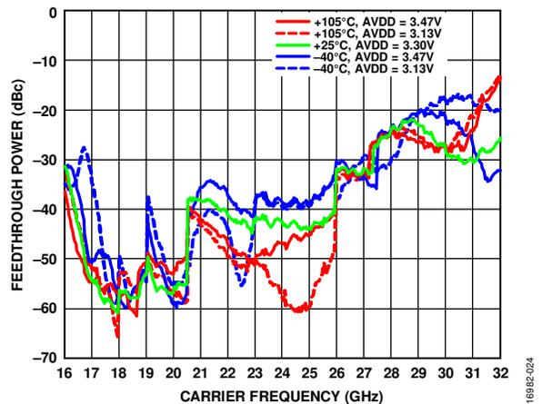
Figure 24. RF32P and RF32N VCO x 3 Feedthrough, De-Embedded Board and Cable Measurement, Combined Using Balun
