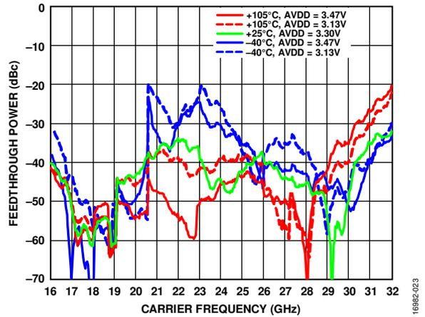
Figure 23. RF32P and RF32N VCO x 2 Feedthrough, De-Embedded Board and Cable Measurement, Combined Using Balun
