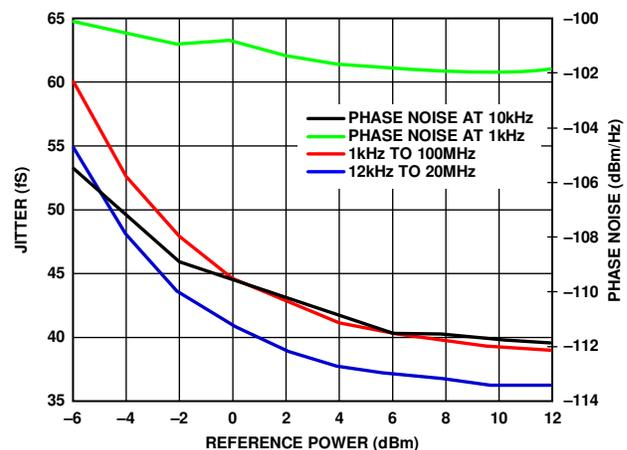
Figure 33. Jitter and Phase Noise,  $f_{PFD} = 250\ MHz$
