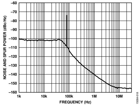
Figure 18. Fractional-N Spur Performance,  $R_{F_{OUT}A+} = 2.591$  GHz,  $R_{F_{IN}} = 122.88$  MHz,  $P_{FD} = 61.44$  MHz, Output Divide by 2 Selected, Loop Filter Bandwidth = 40 kHz, Channel Spacing = 20 kHz
