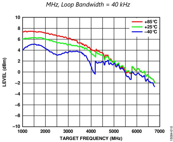
Figure 10. Output Power vs. Frequency,  $RF_{outA+}/RF_{outA-}$  (7.4 nH Inductors, 10 pF AC Coupling Capacitors, Board Measurement)
