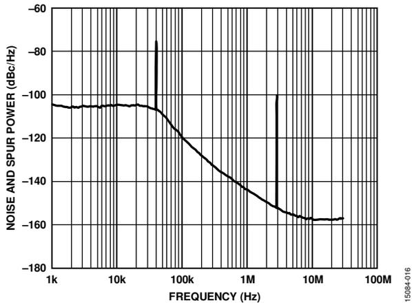
Figure 16. Fractional-N Spur Performance, GSM1800 Band,  $R_{F_{OUT}A+} = 1550.2$  MHz,  $R_{F_{IN}} = 122.88$  MHz,  $P_{FD} = 61.44$  MHz, Output Divide by 4 Selected, Loop Filter Bandwidth = 40 kHz, Channel Spacing = 20 kHz
