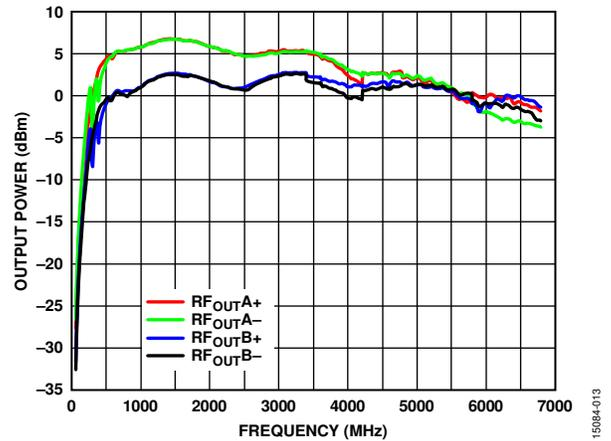
Figure 13.  $RF_{outA+}/RF_{outA-}$  Power vs.  $RF_{outB+}/RF_{outB-}$  Power (7.4 nH Inductors, 10 pF AC Coupling Capacitors, Board Measurement)
