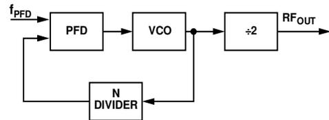
Figure 42. Loop Closed Before Output Divider
