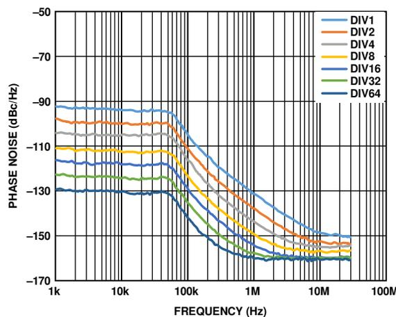
Figure 9. Closed-Loop Phase Noise,  $R_{FoutB+}$  (100 nH Inductors), Fundamental VCO and Dividers, VCO = 6.8 GHz, PFD = 61.44 MHz, Loop Bandwidth = 40 kHz
