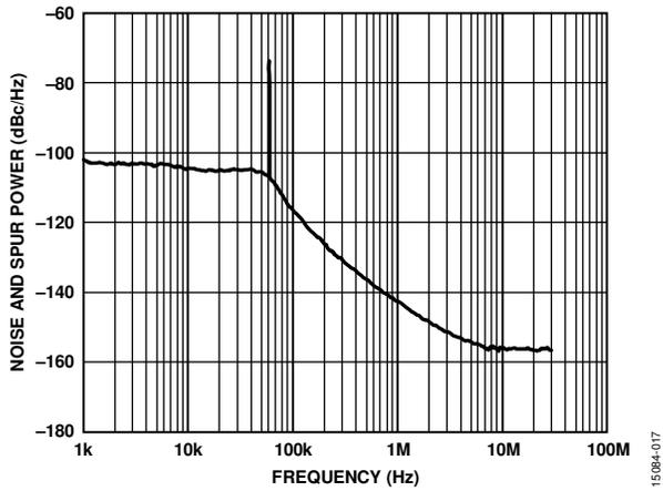
Figure 17. Fractional-N Spur Performance, W-CDMA Band,  $R_{F_{OUT}A+} = 2113.5$  MHz,  $R_{F_{IN}} = 122.88$  MHz,  $P_{FD} = 61.44$  MHz, Output Divide by 2 Selected, Loop Filter Bandwidth = 40 kHz, Channel Spacing = 20 kHz
