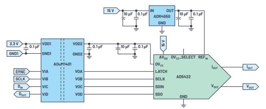
Figure 1. Simplified example circuit for isolated control of an analog output stage using the AD5422 and the ADuM1401.
