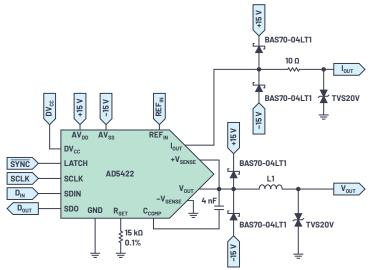
Figure 2. IEC 61000-compliant protective circuits for the outputs of the AD5422.
