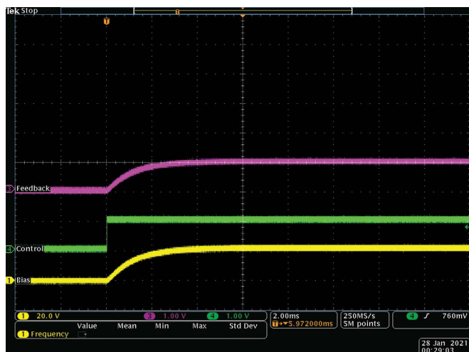
Figure 8. Step response (0 V to 1 V control input).
