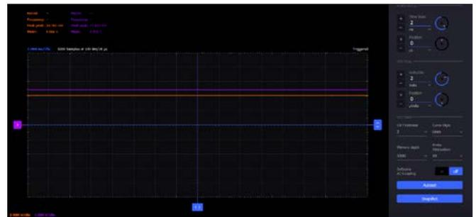
Figure 16. Unipolar and bipolar output voltages for FFF input.
