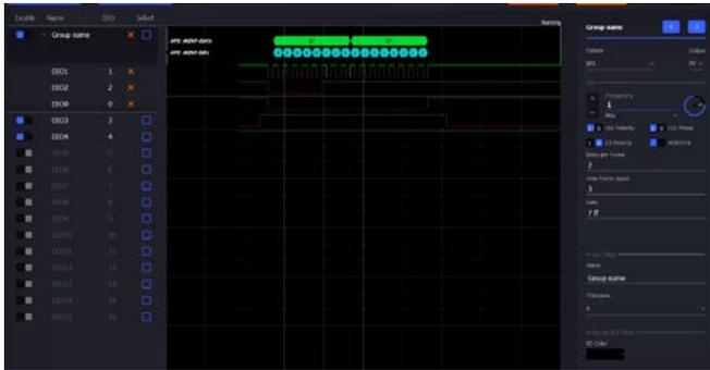
Figure 10. Pattern Generator signals setup.
