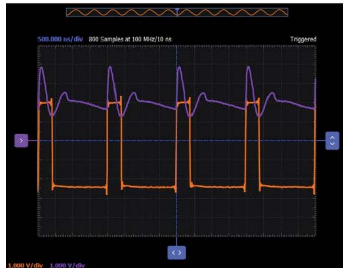
Figure 5. Channel 2 measuring the voltage across emitter resistor R3.
