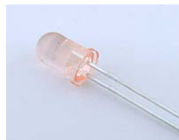
Figure 2. QED123 infrared LED.
