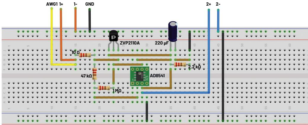
Figure 2. Active half wave rectifier with a self-powered op amp breadboard circuit.
