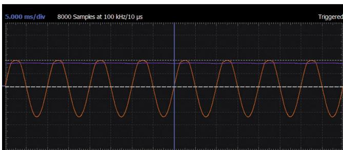
Figure 3.  $V_{OUT}$  and  $V_{IN}$  at 220  $\mu\text{F}$  capacitor in a Scopy plot.
