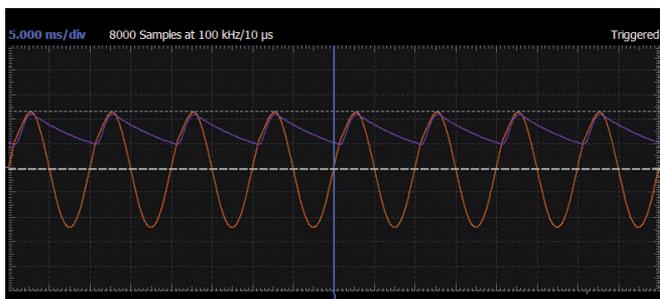
Figure 4.  $V_{OUT}$  and  $V_{IN}$  at 4.7  $\mu\text{F}$  capacitor in a Scopy plot.
