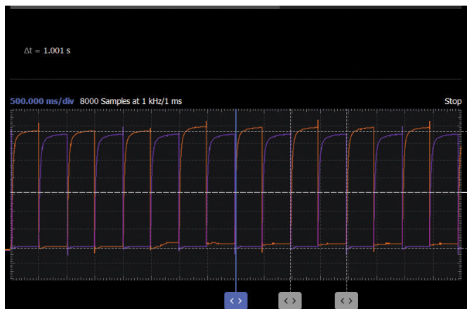
Figure 3. Astable multivibrator interval at 47 \mu\text{F} capacitor.
