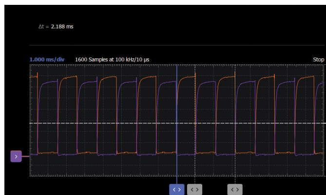
Figure 4. Astable multivibrator interval at 0.1 \mu\text{F} capacitor.
