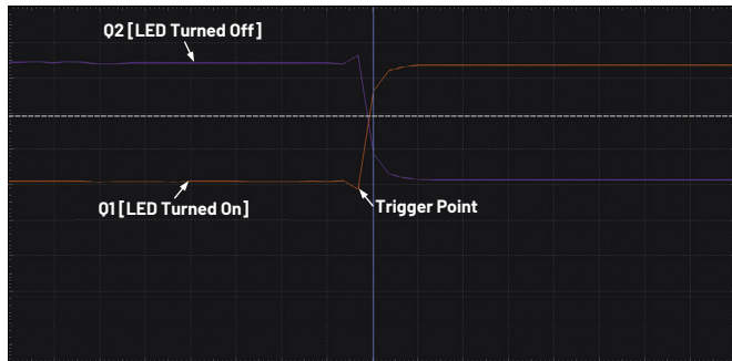
Figure 7. Monostable multivibrator behavior on trigger.
