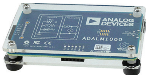
Figure 7. Source measurement unit ADALM1000 from Analog Devices.
