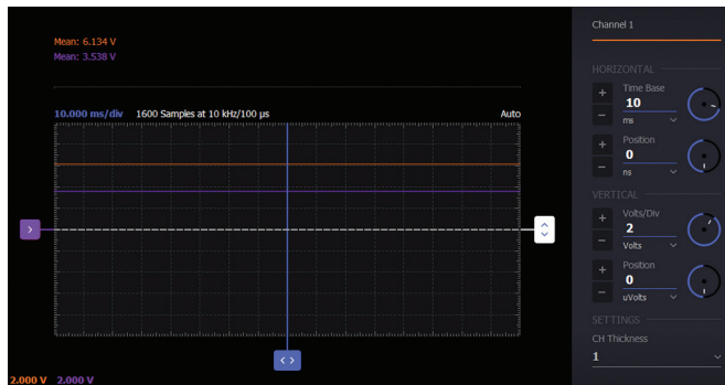
Figure 4. R_L = 10 k \Omega Zener diode regulator waveform.
