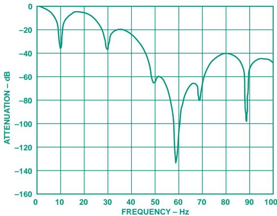
Figure 3. Filter profile showing simultaneous 50 Hz and 60 Hz rejection nulls with sinc<sup>3</sup> filter control word of 69.
