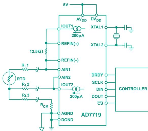
Figure 5. 3-wire RTD measurement using the AD7719.
