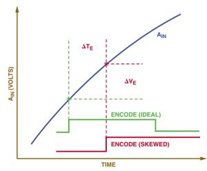
Figure 3. Voltage error due to encode/clock skew.
