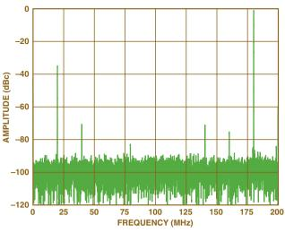
Figure 5. Typical two-converter interleaved FFT plot.
