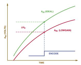
Figure 2. Voltage error due to gain mismatch.
