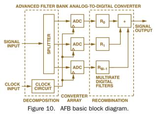
By using a unique multirate FIR filter structure, AFB can be easily implemented into a convenient digital hardware platform, such as an FPGA or CPLD. The FIR coefficients are calculated using a patented method that involves starting with the equations seen in Figure 9, and then applying a variety of advanced mathematical techniques to solve for the digital calibration transfer function.
