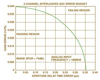
Figure 7. Error budget: 12-bit, 2-channel, 180-MHz input.
