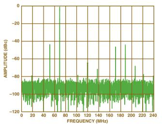
Figure 6. Typical four-converter interleaved FFT plot.
