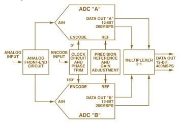
Figure 8. Functional diagram of a traditional time-interleaved ADC.
