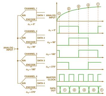
Figure 1. Four-channel time-interleaved ADC system.
