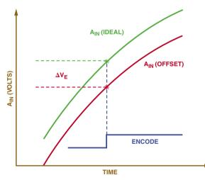
Figure 4. Voltage error due to offset mismatch.
