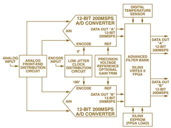
Figure 11. AD12400 block diagram.
