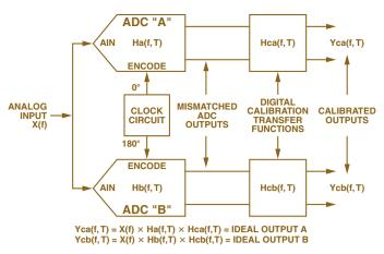
Figure 9. Example of digital post-processing architecture.
