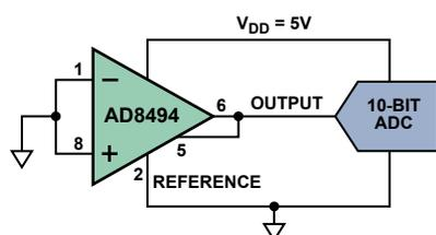
Figure 1. Simple thermometer.
