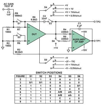
Figure 1. Basic op amp measurement circuit.
