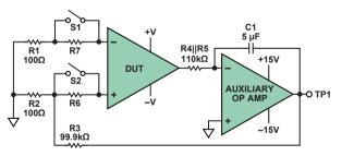
Figure 3. Offset and bias current measurement.
