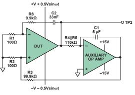
Figure 9. AC PSRR measurement.
