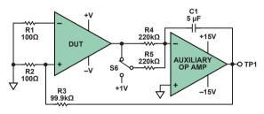
Figure 4. DC gain measurement.
