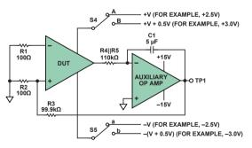
Figure 7. DC PSRR measurement.
