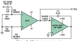
Figure 5. AC gain measurement.
