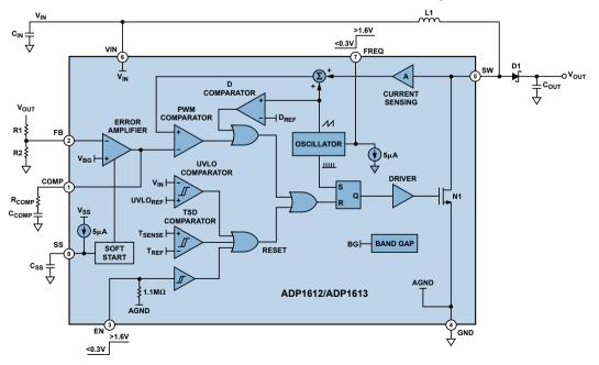
Figure A. ADP1612/ADP1613 functional block diagram.
