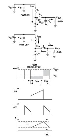
Figure 2. Buck converter topology and operating waveforms.
