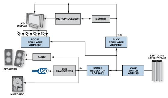
Figure 1. Typical low-power portable system.
