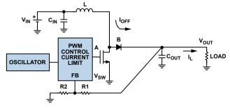
Figure 3. Boost regulator integrates oscillator, PWM control loop, and switching FETs.
