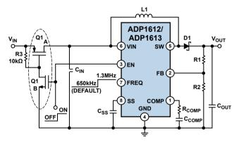
Figure 4. ADP1612/ADP1613 typical applications circuit.
