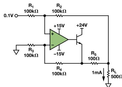
Figure 3. Example circuit for  $I_{OUT} = 1 \text{ mA}$ .
