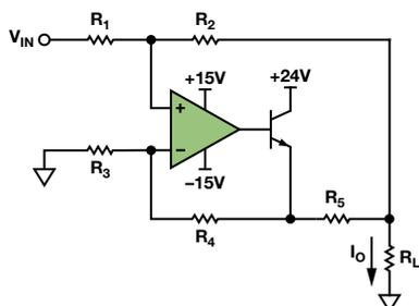
Figure 1. Improved Howland current source drives grounded loads.
