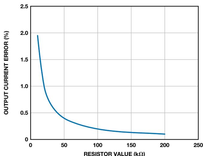
Figure 2. Relationship between  $R_1$  and output current accuracy.
