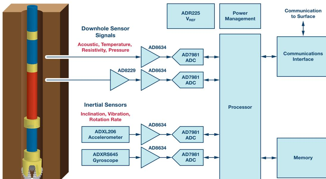
Figure 1. Downhole instrument data acquisition signal chain.
