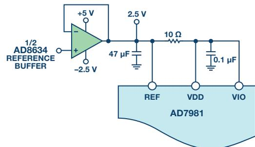
Figure 6. Supplying ADC from reference buffer.
