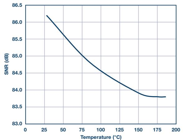
Figure 12. SNR over temperature, 1 kHz input tone, 580 kSPS.
