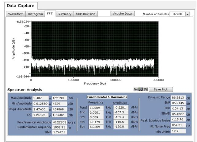
Figure 11. AC performance with 1 kHz input tone, 580 kSPS, 25°C.
