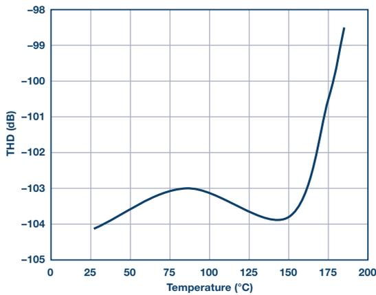
Figure 13. THD over temperature, 1 kHz input tone, 580 kSPS.
