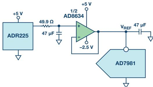
Figure 5. SAR ADC reference buffer and RC filter.
