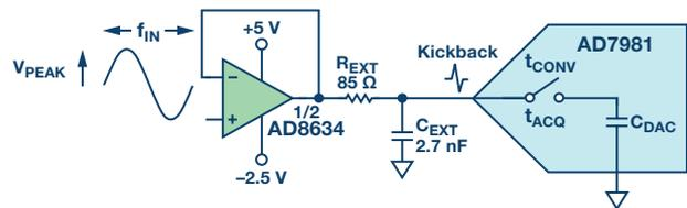
Figure 4. ADC front-end amplifier circuit.
