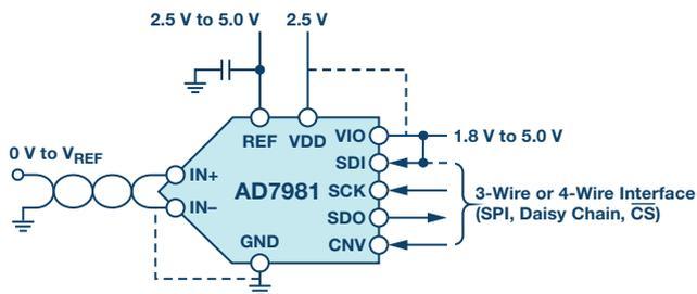
Figure 3. AD7981 application diagram.
