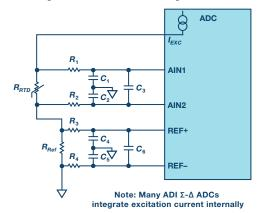
Figure 2. Typical 4-wire RTD ratiometric measurement circuit.
