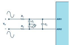
Figure 4. Differential mode low-pass filter.
