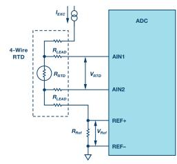
Figure 1. 4-wire RTD ratiometric measurement circuit.
