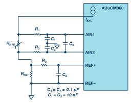
Figure 7. ADuCM360 analog front-end circuit for RTDs measurement.
