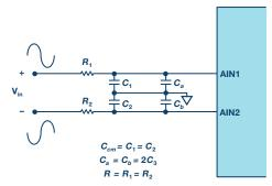
Figure 5. Differential mode low-pass filter equivalent circuit.
