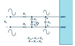
Figure 3. Common-mode low-pass filter.
