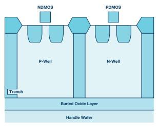
Figure 6. Trench isolated process.
