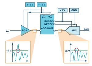
Figure 11. Data acquisition application example.
