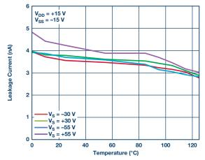
Figure 8. ADG5248F overvoltage leakage current vs. temperature.
