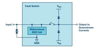
Figure 5. Fault protected switch architecture.
