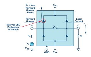
Figure 1. Overvoltage current path.
