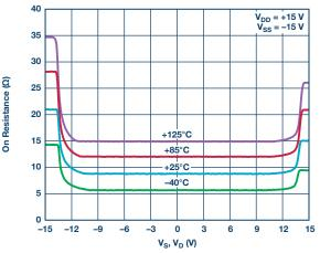
Figure 7. Fault protected switch on resistance.
