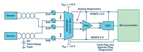
Figure 10. Process control application example.
