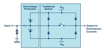
Figure 4. Traditional switch architecture with external discrete protection.
