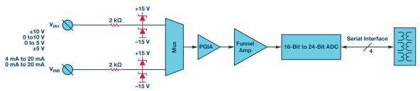
Figure 3. Discrete protection solution.
