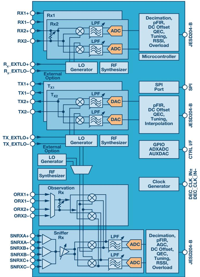
Figure 4. AD9361 and AD9371 block diagrams.
