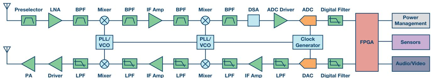
Figure 1. Basic superheterodyne architecture.
