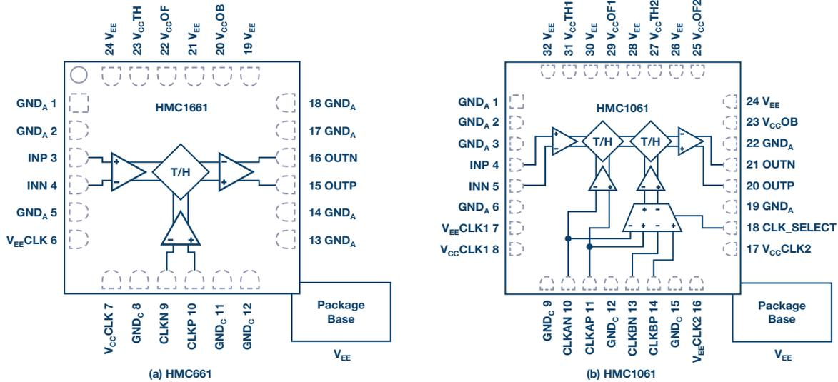
Figure 1. Track-and-hold topologies: (1a) single rank, (1b) dual rank.
