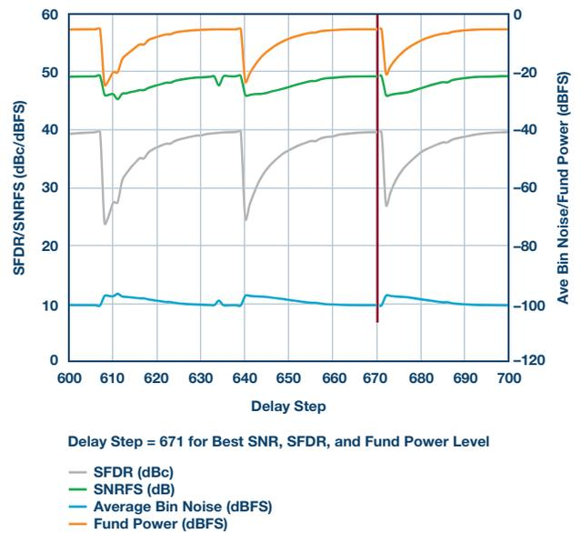
Figure 3b. Mapping results of signal amplitude and SFDR performance over each delay setting (zoomed in).
