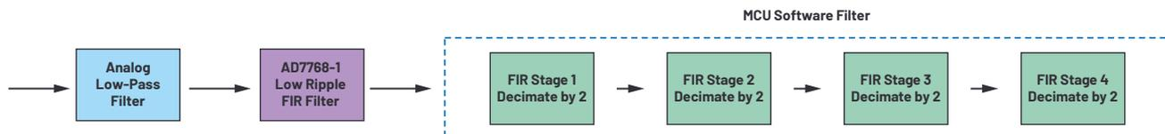
Figure 4. MCU post-FIR filter stages.
