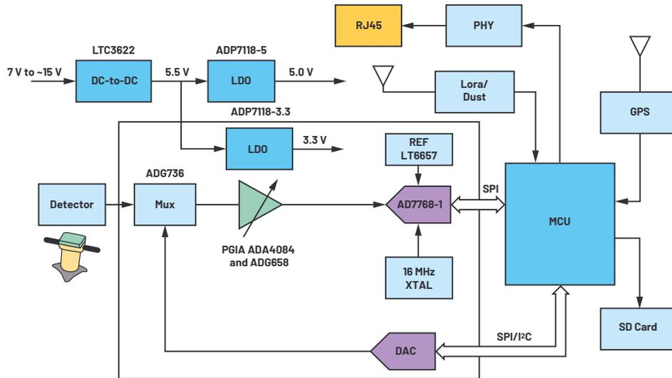
Figure 2. ADA4084-2 PGA and AD7768-1 plus MCU filtering signal chain solution.
