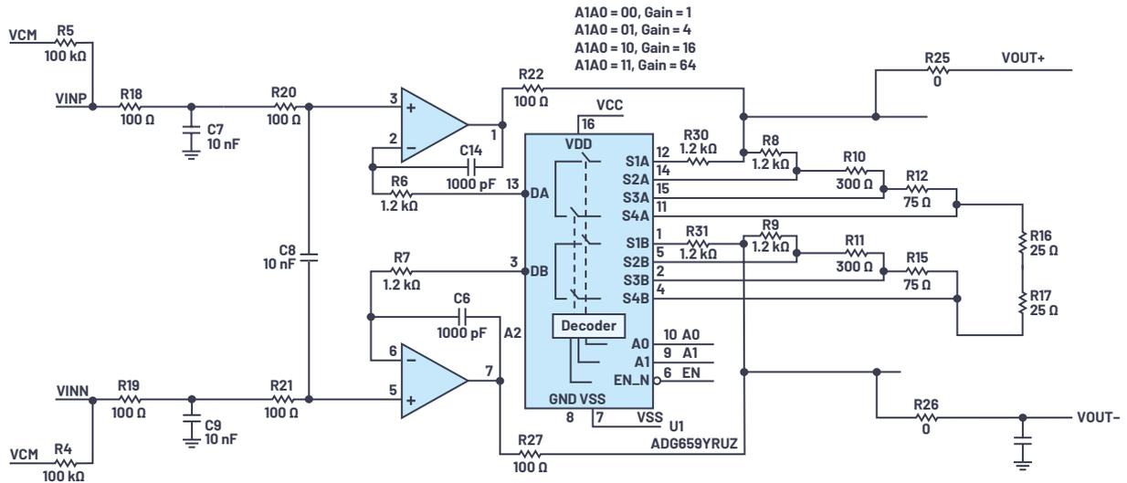
Figure 8. A PGA to drive the LTC2500-32.
