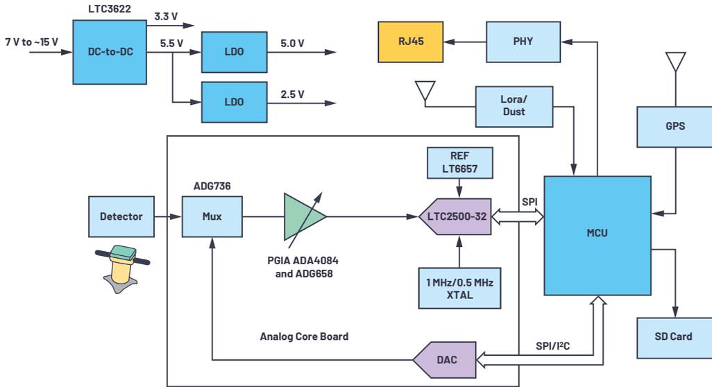
Figure 5. ADA4084-2 PGA and LTC2500-32 signal chain solution.
