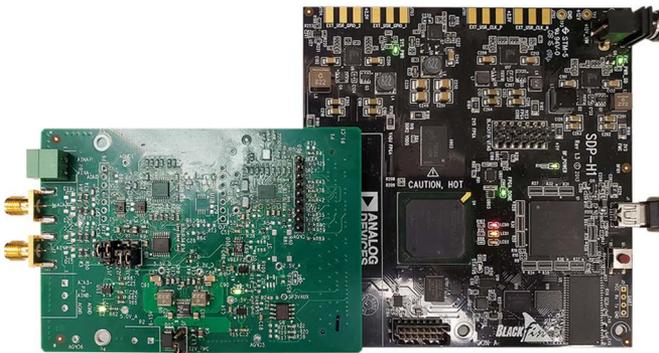
Figure 9. ADA4084-2 PGA and AD7768-1 evaluation board solution.
