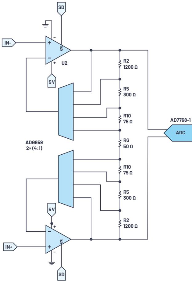
Figure 7. Block diagram of a discrete PGIA.
