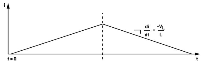
Figure 1. The output current of a buck converter.
