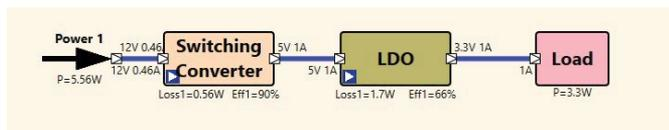
Figure 3. A block diagram of an LDO regulator in postregulation.
