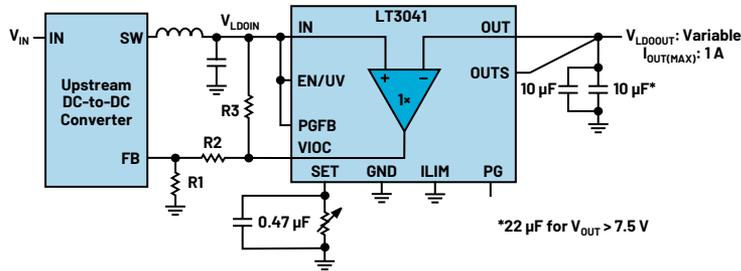
Figure 8. A variable load circuit configuration.
