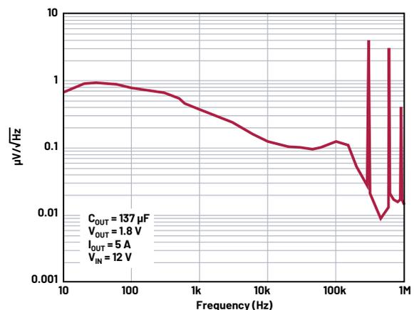
Figure 2. The voltage noise of a switching converter.
