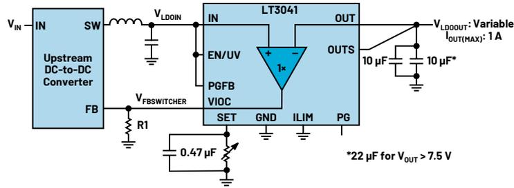
Figure 6. A typical application circuit.
