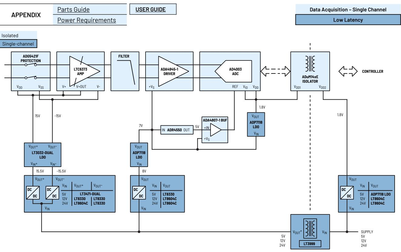
\*The actual output voltage of LT3999 isolated converter depends primarily on the turns ratio of the transformer used. See LT3999 datasheet for details.
