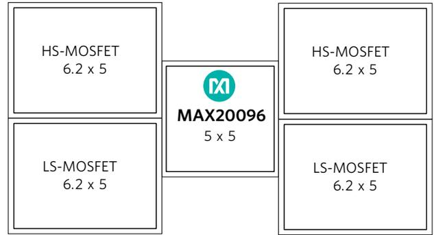
Figure 5. Synchronous Rectification Solution Footprint (149mm<sup>2</sup>)
