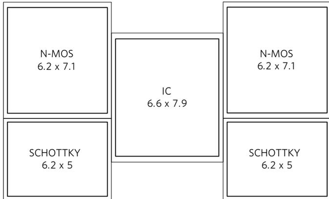
Figure 3. Non-Synchronous Rectification Solution Footprint (264mm<sup>2</sup>)
