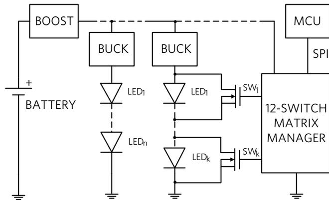
Figure 7. LED Driver Solution With 12-Switch Matrix Manager
