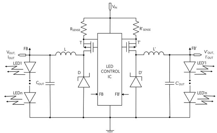
Figure 2. Typical Dual Controller Non-Synchronous Rectification Solution
