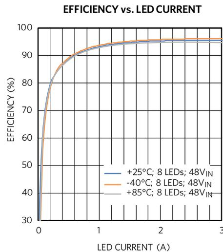
Figure 6. LED Driver Solution Efficiency vs. Load Current
