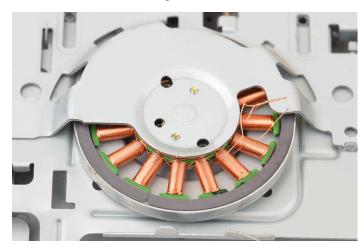
Figure 2. BLDC with Removed Upper Cover and Magnet Rotor
