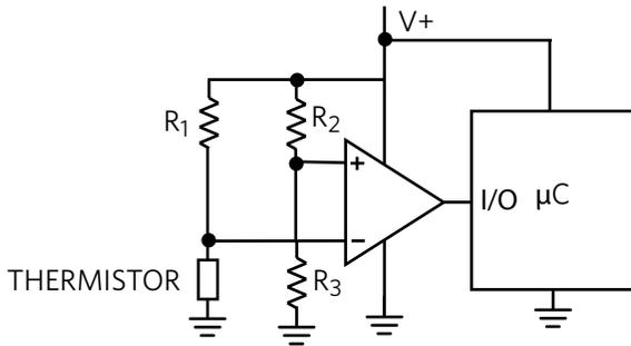
Figure 3. Temperature Monitoring Using a Comparator
