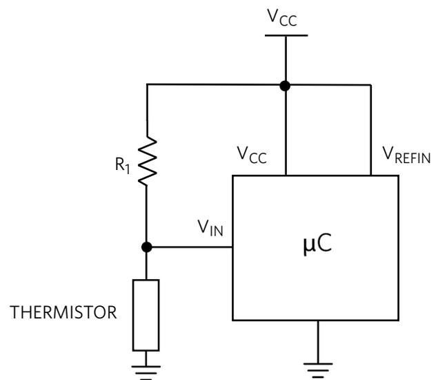
Figure 2. Temperature Monitoring Circuit Using a Thermistor
