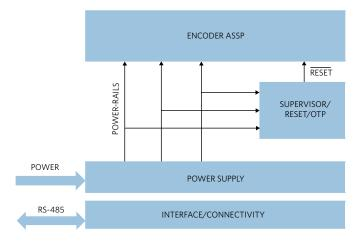
Figure 4. Encoder ASSP Power Rails Control
