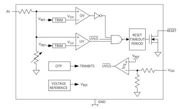
Figure 6. MAX16132 µP Supervisor Block Diagram
