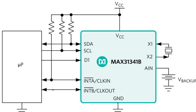
Figure 3. MAX31341B RTC Typical Operating Circuit
