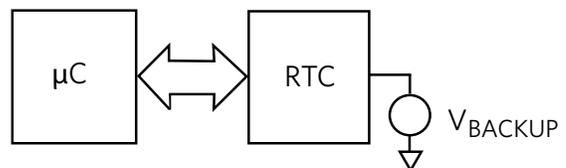
Figure 2. External RTC Interfaced to a Microcontroller
