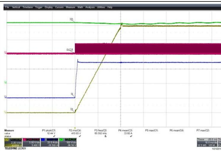
Figure 11 - Startup at 400VDC, 600W load (software PSON)
