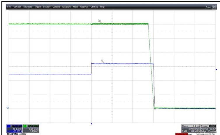
Figure 12 - 65A load (Action to shutdown after ~10ms)
