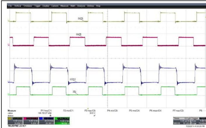
Figure 14 – The PWM timing of LLC converter and SR @  $I_o=20A$
