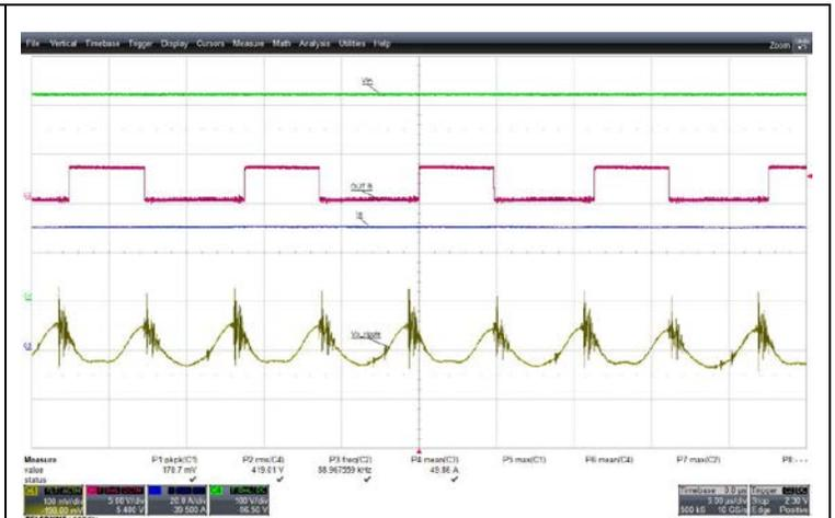
Figure 17 – Output voltage AC coupled 400VDC, 50A, 100mV/div, 5us/div.
