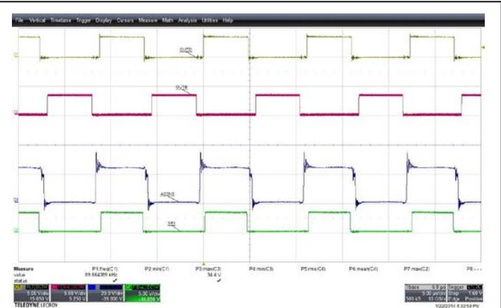
Figure 15 – The PWM timing of LLC converter and SR @  $I_o=50A$
