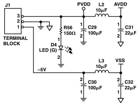
Figure 14. Schematic-Power Supply
