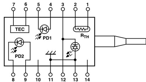
Figure 4. Laser Module Pin Assignment (reference: Fujitsu Quantum Devices, FLD5F6CA Data Sheet)
