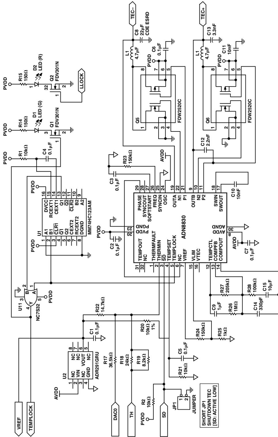
Figure 12. Schematic-TBC Control
