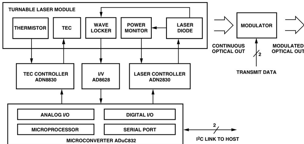
Figure 1. Typical Block Diagram of Optical Transmitter with DFB Laser Module
