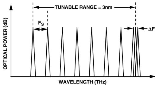
Figure 2c. Frequency Slots and Allowable Frequency Deviation
