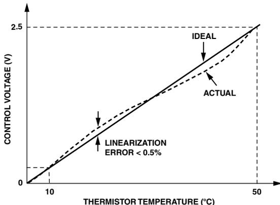
Figure 7. V-to-Temperature Characteristic
