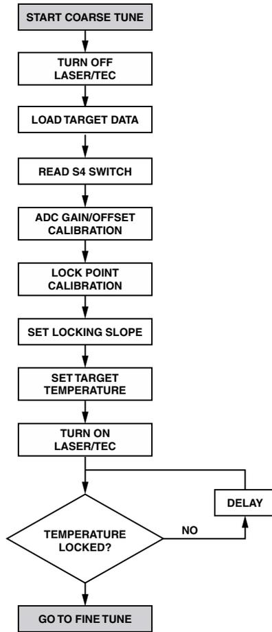
Figure 9. Coarse Tuning Flow Chart
