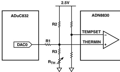
Figure 6. Application Circuit Using DAC Control Voltage
