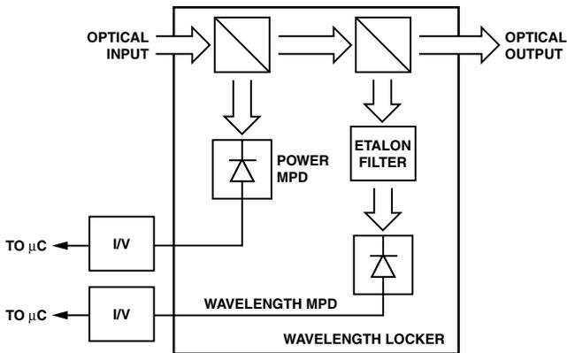
Figure 2a. Wavelength Locker Block Diagram
