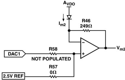
Figure 5. I/V Conversion Circuit
