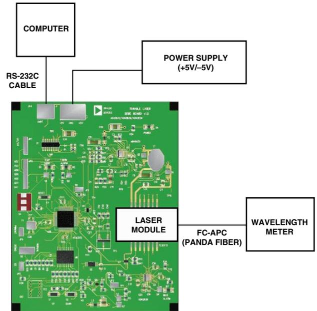
Figure 3. Demo Board Setup
