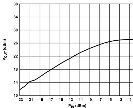
Figure 8.  $P_{OUT}$  vs.  $P_{IN}$  (433.92 MHz Input)
