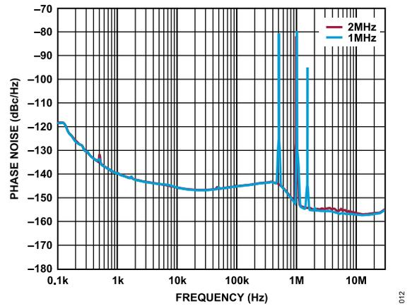
Figure 12. CN0551 Phase Noise using Different LTM4693 Switching Frequencies (1 MHz and 2 MHz)
