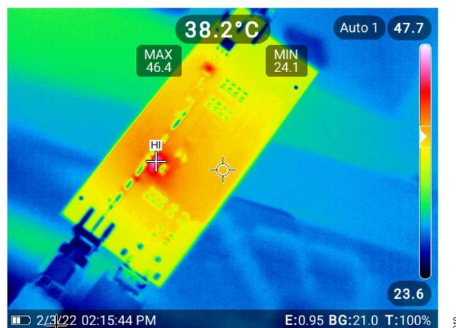
**Figure 10. CN0551 Thermal Performance (RF Input Power = -10 dBm)**
