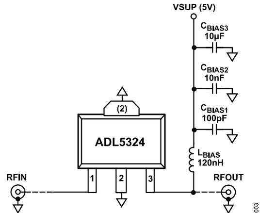
Figure 3. ADL5324 DC Bias Inductor and Capacitors
