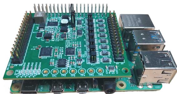
Figure 14. EVAL-CN0554-RPIZ Attached to the Raspberry Pi
