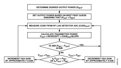
Figure 4. Operation of Transmitter After Calibration
