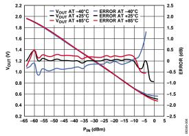
Figure 8. Multipoint Calibration Extends Detector Range and Can Improve Linearity but at the Cost of a More Complex Calibration Procedure
