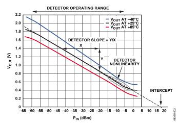
Figure 2. Transfer Function ( $V_{OUT}$  vs.  $P_{IN}$ ) of a Log-Responding RF Power Detector with Temperature Drift Exaggerated for Illustrative Purposes
