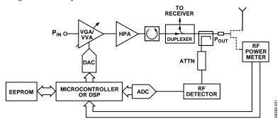
Figure 1. Typical RF Power Amplifier with Integrated Transmit Power Control (An integrated RF power detector provides continuous feedback on the current level of power being transmitted.
