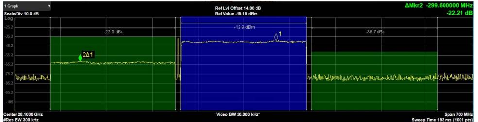
Figure 10. 200 MHz 5G NR Signal on MxFE-ADMV1018 Board. The Image is at -22.5 dBc
