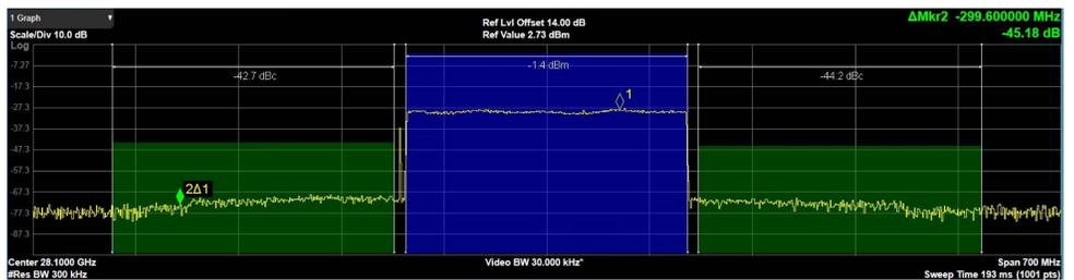
Figure 11. 200 MHz 5G NR Signal on MxFE-ADMV1018 Board. The Image is -42.7 dBc Using ORx Path That has been Calibrated with CW Tones
