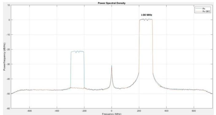
Figure 8. Image Rejection on Downconverter ADMV1018: A) 100 MHz Centered at 250 MHz at the Output of the Downconverter ADMV1018 Without Applying the QEC Algorithm, B) the Same 100 MHz After Applying the QEC Algorithm. Note That the Image is Suppressed (IRR is 50 dB)
