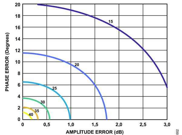
Figure 2. Contours for the IRR (in dB) vs. Gain and Phase Imbalance
