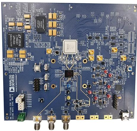
Figure 3. Data Converter (AD9988) + 5G Upconverter and Downconverter ADMV1018 (UDC) Used for ZIF QEC
