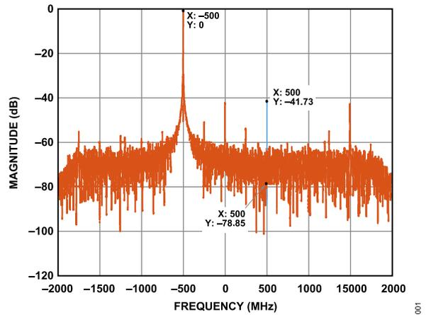
Figure 1. Illustration for the Image Frequency: A Carrier Wave Tone at -500 MHz and Its Image at 500 MHz
