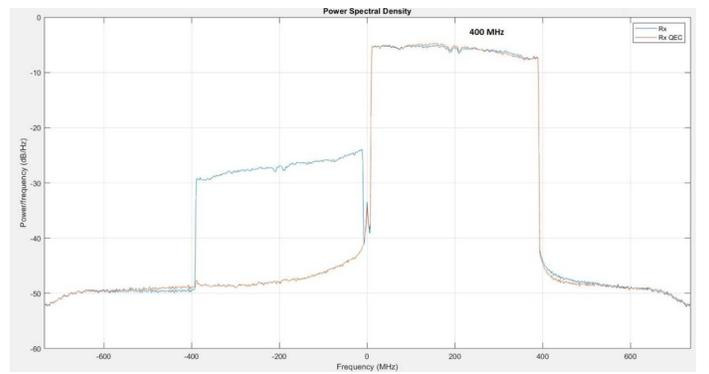
**Figure 9. Image Rejection on Upconverter ADMV1018: A) 400 MHz Centered at 200 MHz at the Output of Downconverter ADMV1018 Without Applying the QEC Algorithm, B) the Same 400 MHz After Applying the QEC Algorithm. Note That the Image is Suppressed (IRR is About 45 dB)**
