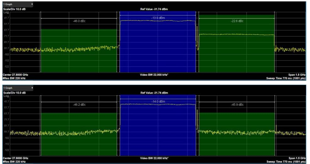
Figure 7. Image Rejection on Upconverter ADMV1018: A) 400 MHz Centered at 27.8 GHz at the Output of ADMV1018 Without Applying the QEC Algorithm, B) the Same 400 MHz After Applying the QEC Algorithm. Note That the Image is Suppressed (IRR is 45.9 dB)
