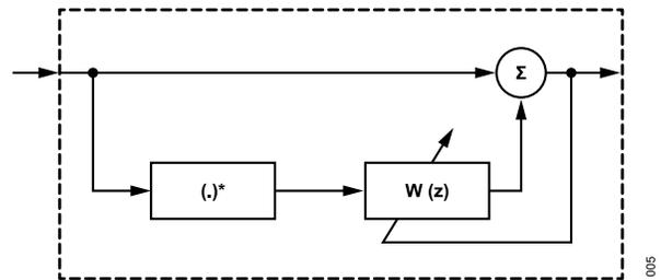
Figure 5. Complex Adaptive Digital Filter Used for QEC
