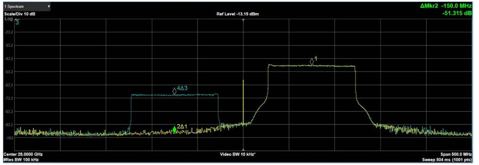
Figure 6. Image Rejection on Upconverter ADMV1018: The Yellow Curve is a 100 MHz NR Signal at 28.150 GHz Captured at the Output of the Upconverter of ADMV1018, the Blue Curve is for the Same Signal When QEC Algorithm is Applied
