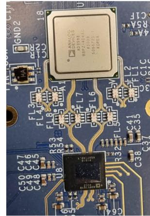
Figure 4. Data Converter (AD9988) + 5G Upconverter and Downconverter Zoomed Photo
