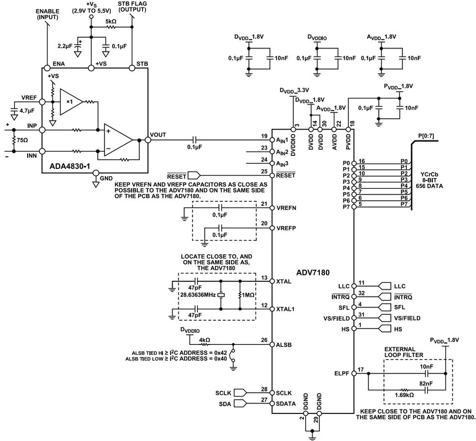
Figure 1. Robust Differential Video Receiver with the ADA4830-1 and the ADV7180 (All Connections and Decoupling Not Shown)
