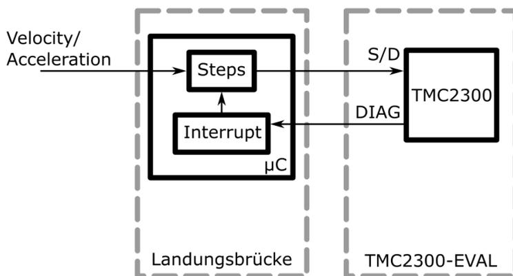
Figure 5: StallGuard System Overview: Motion Controller inside the  $\mu C$
