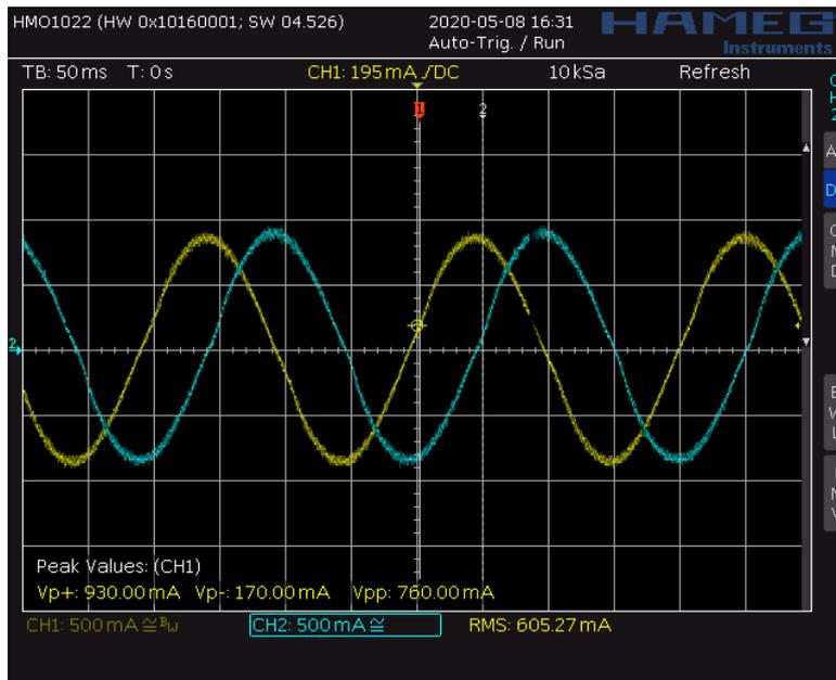
Figure 8: Phase currents with 680mA setting at 50kpps
