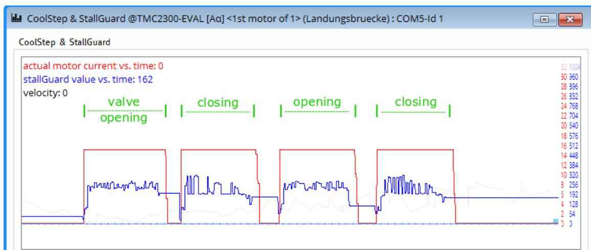
Figure 6: Valve 1 StallGuard value, target velocity: 100kpps, velocity threshold: 90kpps, StallGuard threshold: 50
