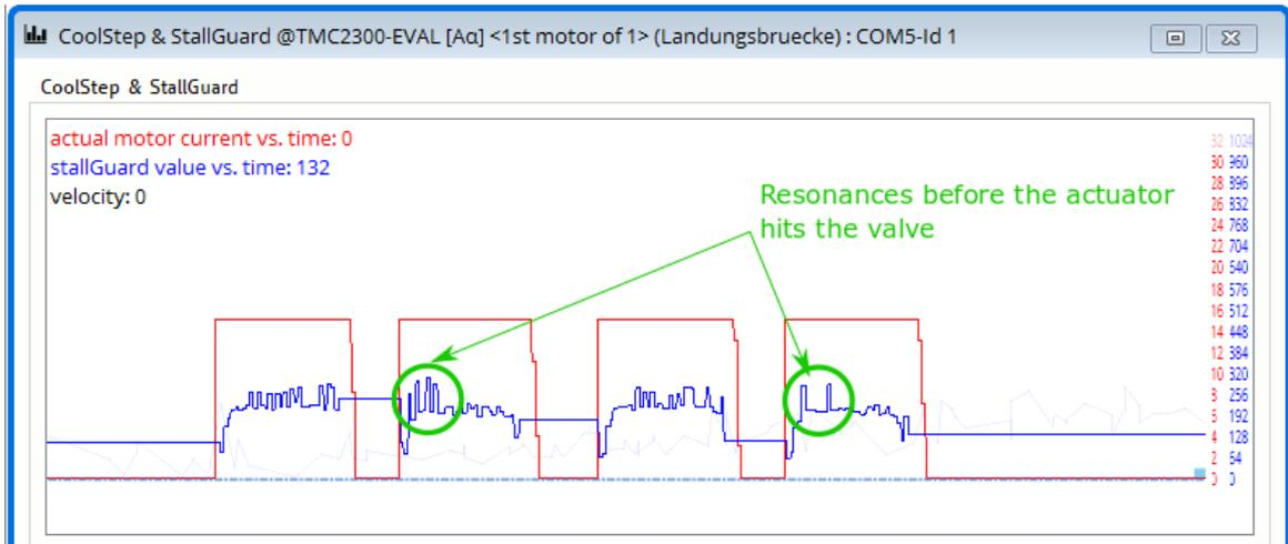
Figure 7: Valve 2 StallGuard value, target velocity: 100kpps, velocity threshold: 90kpps, StallGuard threshold: 50
