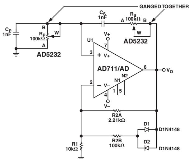
Figure 1. Programmable Wien-Bridge Oscillator with Amplitude Stabilization
