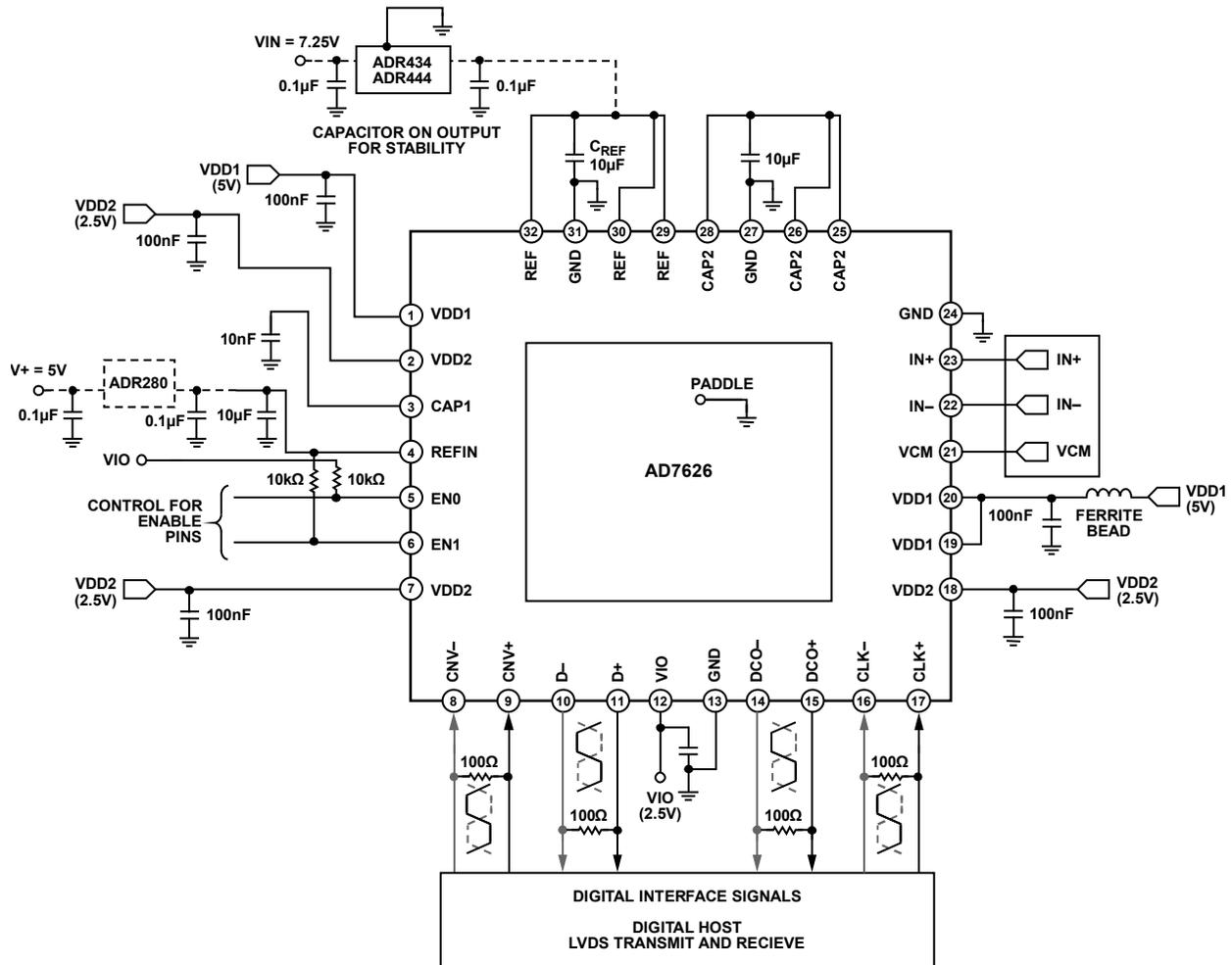
Figure 4. Typical Connection Diagram for AD7626 Showing Decoupling and LVDS Interface Connections
