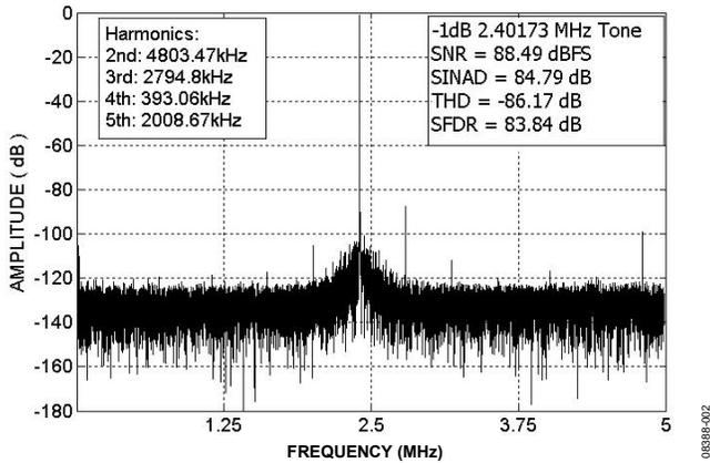
Figure 2. *AD7626* Output, 64,000 Point, FFT Plot,  $-1$  dBFS Amplitude, 2.40173 MHz Input Ton, 10,000 MSPS Sampling Rate
