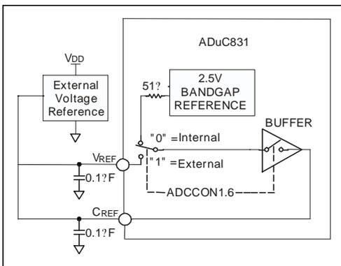
**Using the internal reference:** On the ADuC812 to use the internal reference as a reference to external circuitry the Vref pin was used. This can be used to maintain compatibility with the ADuC812 however there is a gain error between this and the reference used for the ADC conversions.
