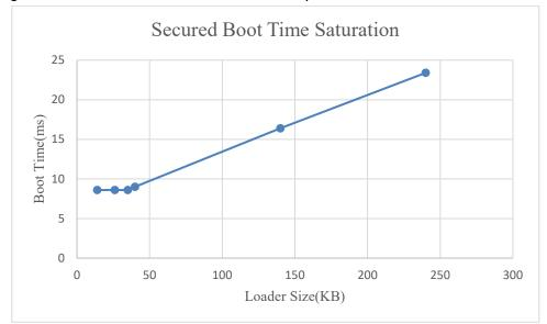
Figure 12: Boot Time Saturation in SPI2 BLp-256 Duel-STR Boot at 62.5 MHZ
