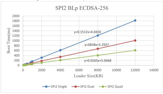
Figure 2: SPI Secured BLp-256 Boot at 62.5 MHz
