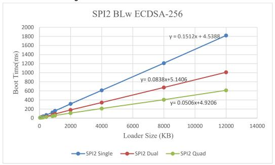
Figure 4: SPI2 BLw-256 Boot at 62.5 MHz
