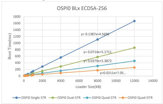
Figure 7: OSPI0 BLx-256 Boot at 62.5 MHz
