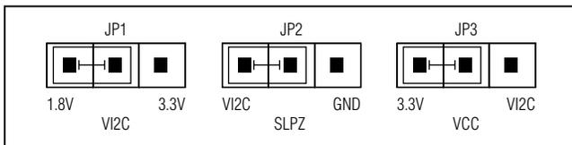
Figure 17. 1.8V I<sup>2</sup>C I/F and 3.3V 1-Wire
