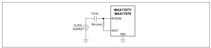
Figure 1. Synchronization to an External Clock
