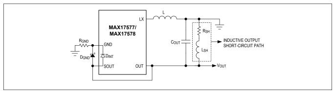
Figure 4. Inductive Output Short-Circuit Protection
