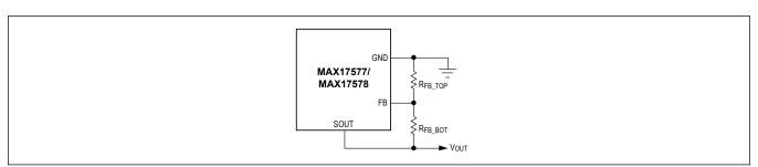
Figure 2. Setting the Output Voltage
