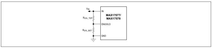
Figure 3. Setting the Input Undervoltage-Lockout
