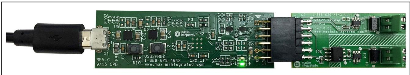
Figure 2. MAX22191PMB# with USB2PMB2# Adapter
