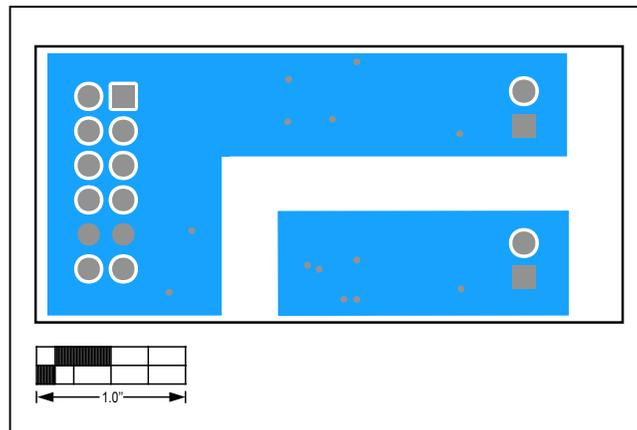
MAX22191PMB# EV Kit PCB Layout—Bottom Layer
