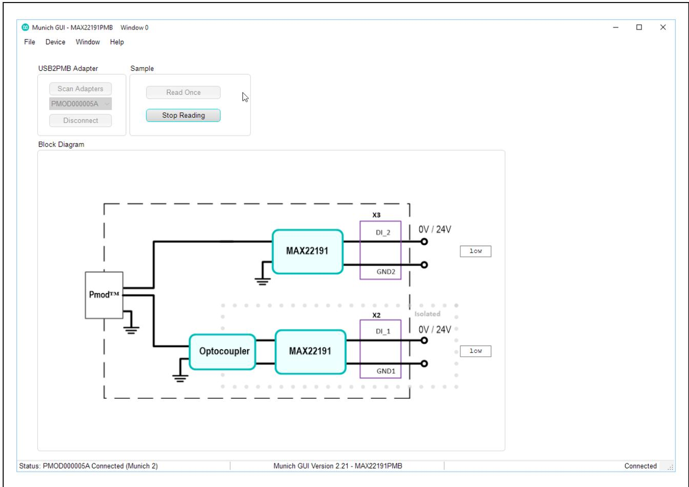
Figure 7a. MAX22191PMB# Software (Munich GUI—Both Inputs Low)
