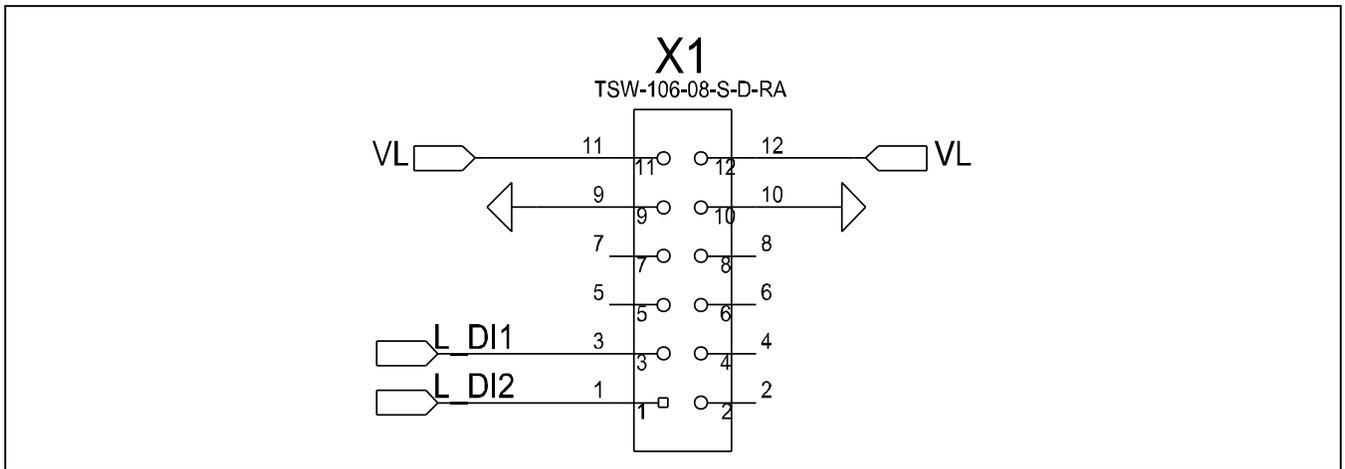
Figure 5. X1 Connector Pin Out
