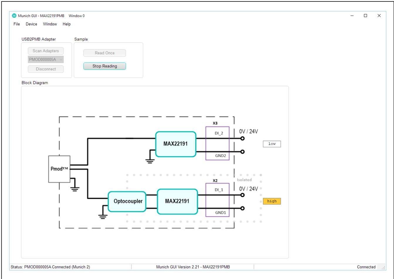
Figure 7b. MAX22191PMB# Software (Munich GUI–Input 2 High)
