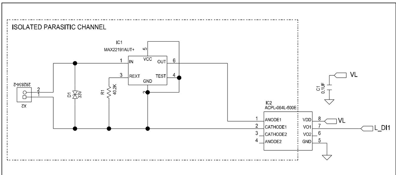
Figure 3. Input 1—Isolated Parasitic Channel
