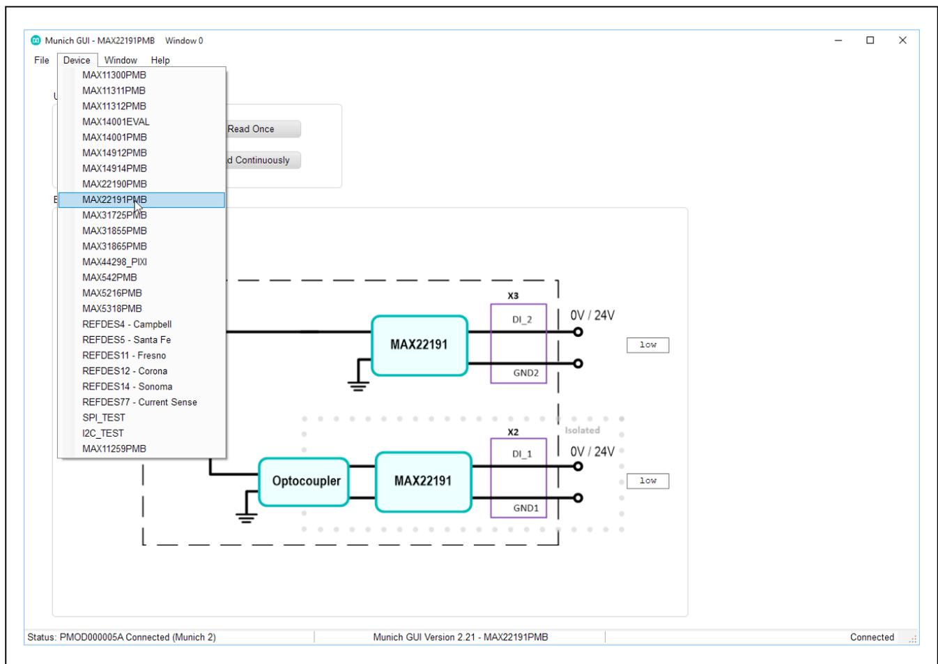
Figure 6. MAX22191PMB# Software (Munich GUI Device Menu)
